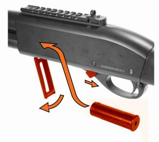
Push the bolt release catch to open the carrier latch and LOAD the shell type magazine.
