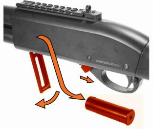
Push the bolt release catch to open the carrier latch and UNLOAD the shell type magazine.
